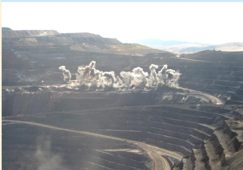
View of a mining blast in progress at an open pit gold mine in Nevada. A pattern of 18-ft holes is drilled on the pit floor (or other intended blast level), loaded with explosives, then blasted to break the rock for mining. Ore and waste are then loaded using electric shovels into 400-ton haul trucks for removal to processing facilities or waste rock repositories. Catchment benches are 60 feet high. T. Bush photo.
