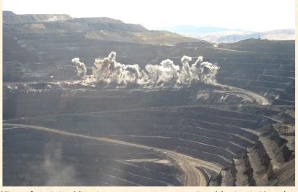
View of a mining blast in progress at an open pit gold mine in Nevada. A pattern of 18-ft holes is drilled on the pit floor (or other intended blast level), loaded with explosives, then blasted to break the rock for • Next Board meeting: June 21, 2011, mining. Ore and waste are then loaded using electric shovels into 400ton haul trucks for removal to processing facilities or waste rock repositories. Catchment benches are 60 feet high. T. Bush photo.
