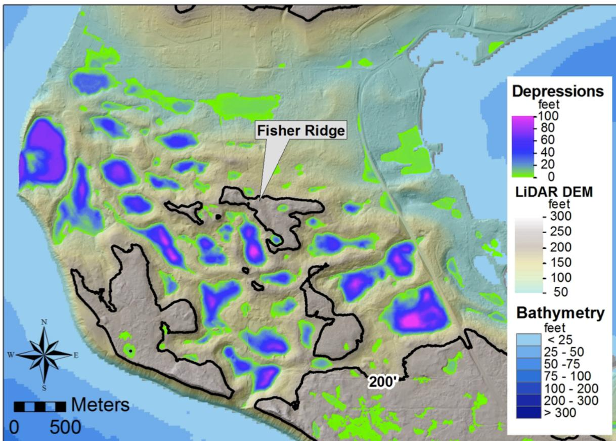
**Figure 8.** Closed depressions in Partridge Gravel near Point Partridge. This lidar map was drafted by H.M. Greenberg (ESS, UW) and has illumination from the northwest at 45 degrees. See text for explanation.
