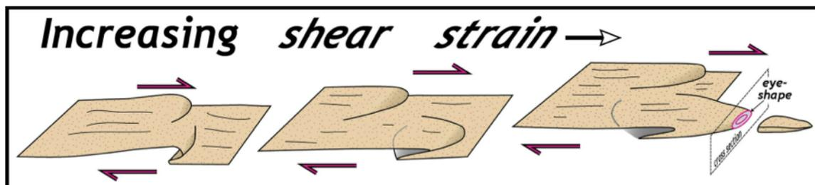
**Figure 10.** Schematic development of sheath folds ([wmblogs.wm.edu](http://wmblogs.wm.edu)). In a material undergoing increasing shear strain with the sense of shear shown by arrows, early folds are distorted as the curved hinges are drawn out into sheaths. The thin black lines represent lineations, which are parallel to the direction of tectonic transport.
