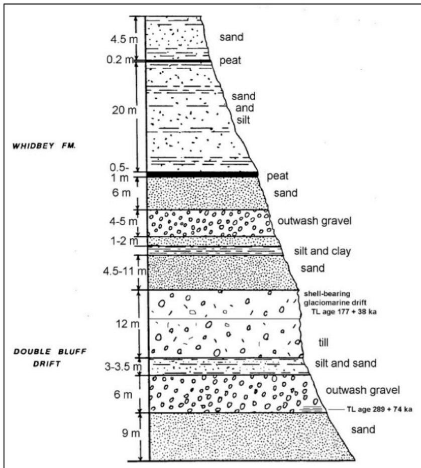
**Figure 3.** Composite stratigraphic section at Double Bluff (Easterbrook, 1994a, fig. 9).
