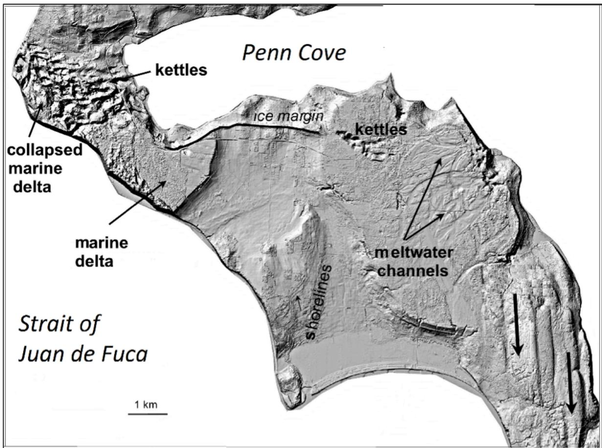
**Figure 6.** Lidar image showing landforms in the Penn Cove area (after Easterbrook, 2003a, fig 8 and Polenz et al., 2005, fig. 1). Vashon drumlins and flutes are the north-south features south of Penn Cove. The outwash and marine deltas are composed of the Partridge Gravel. Still younger marine shorelines are slightly younger than Everson glaciomarine drift (11,700 <sup>14</sup>C yr BP).
