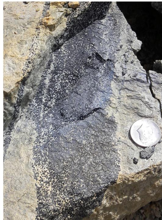
**Figure 10.** A chromite-rich zone (dark area) within the dunite at the Swen Larson Quarry (T. Bush photo). U.S. 50-cent piece coin for scale.
