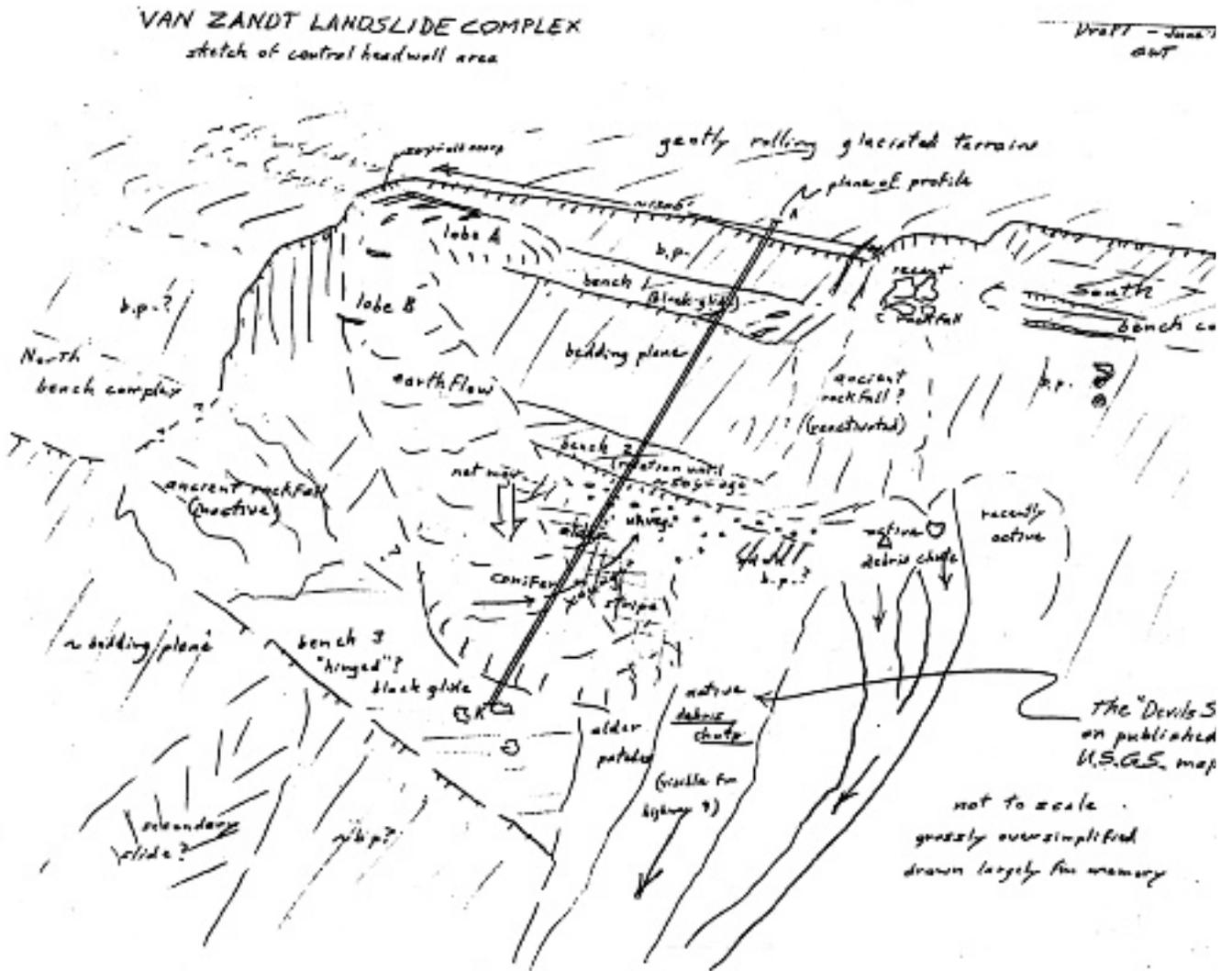
**Figure 11.** Van Zandt landslide complex: oblique field sketch of central headwall area. (G.W. Thorsen, 1987)
