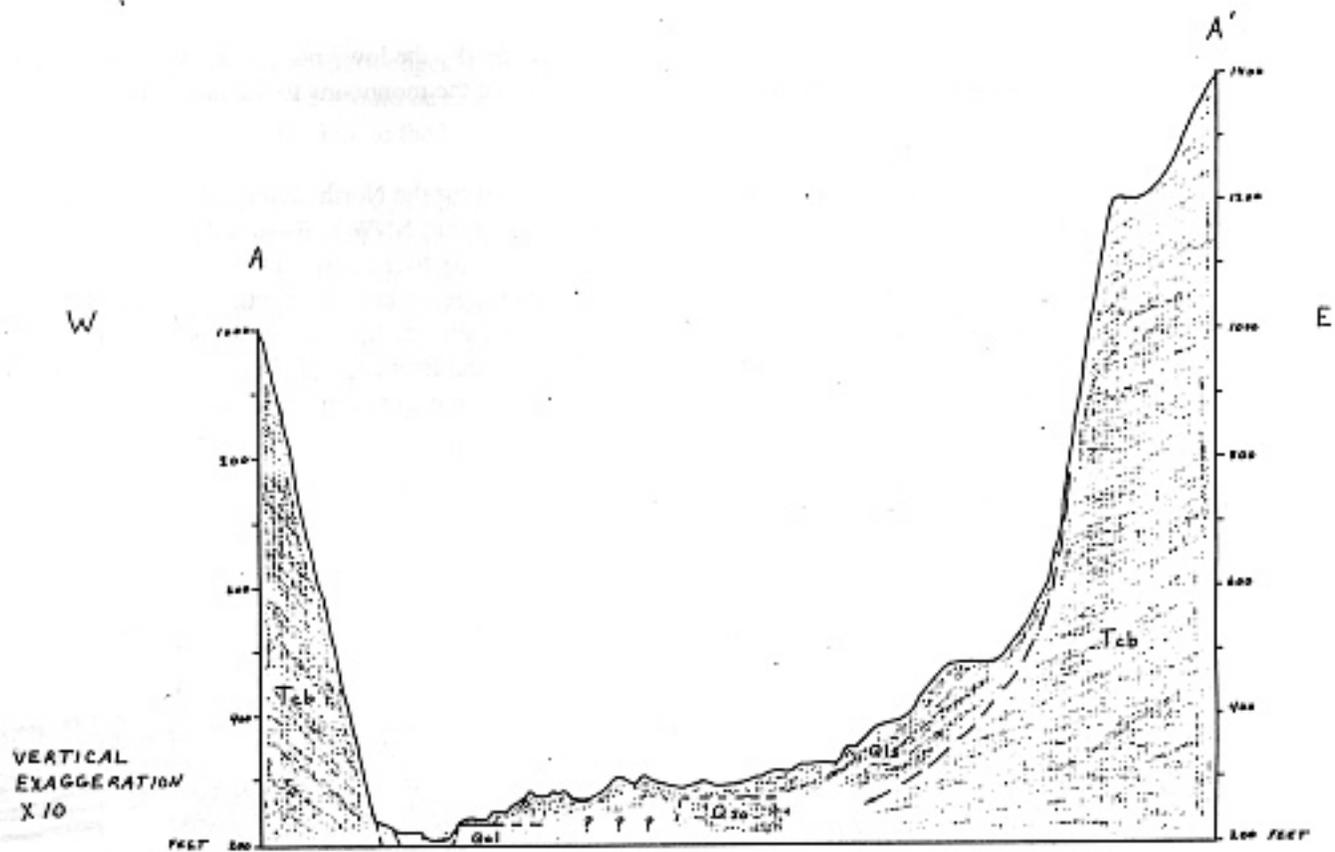
Figure East-west geologic cross-section of the Van Zandt landslide,
